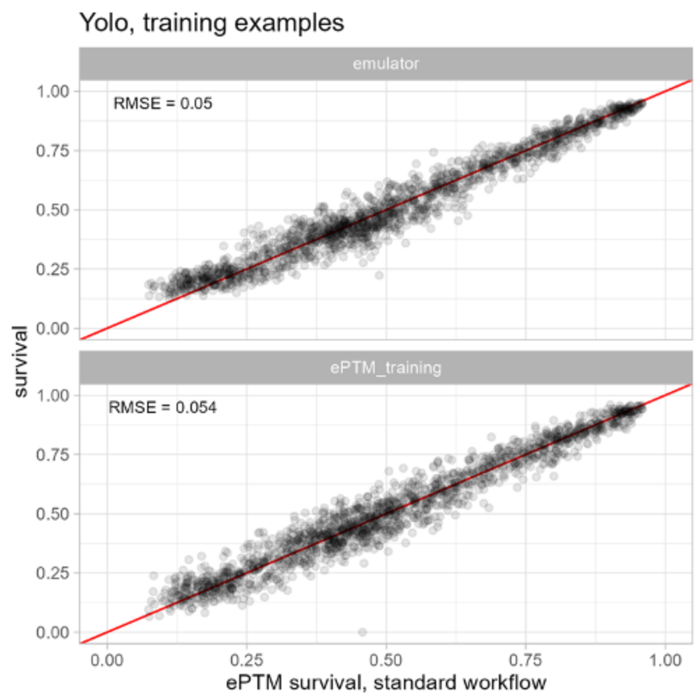
Figure 2. Performance of Yolo emulator on training data (top); inherent run-to-run variability in ePTM outputs at the training points, as shown by comparing independent realizations of the ePTM (bottom)
